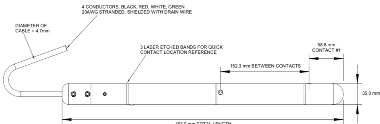
Grounding point / earth stud electrode (3 and 5 electrode FOGRods only, **NOT FOR USE IN SEWAGE**)
